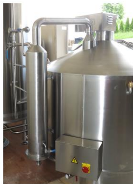
Steam condenser - with energy recuperation
