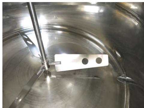
Whirlpool module (tangential entry for the product, liftable stirrer)
