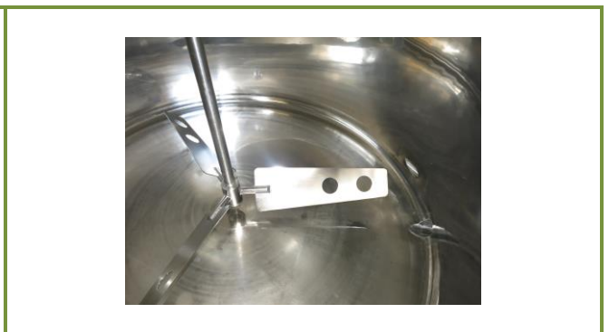
Whirlpool module (tangential entry for the product, liftable stirrer)
